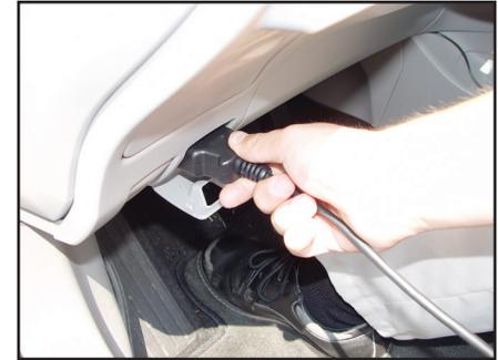
The OBD connector is typically found under your dash near your steering wheel column.
